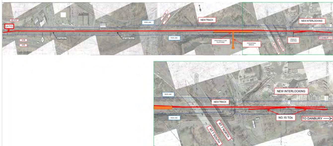
FIGURE 57: SCHEMATIC LAYOUT OF DANBURY FAIR DOUBLE TRACK EXTENSION
