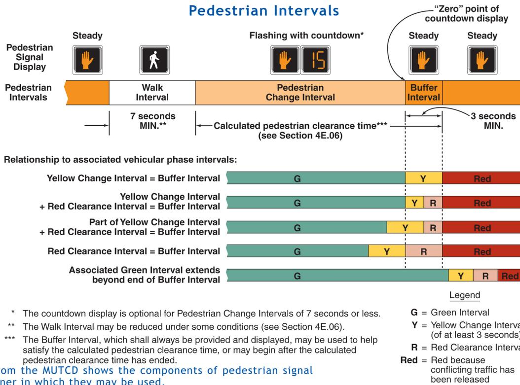
The above figure from the MUTCD shows the components of pedestrian signal timing and the manner in which they may be used.
