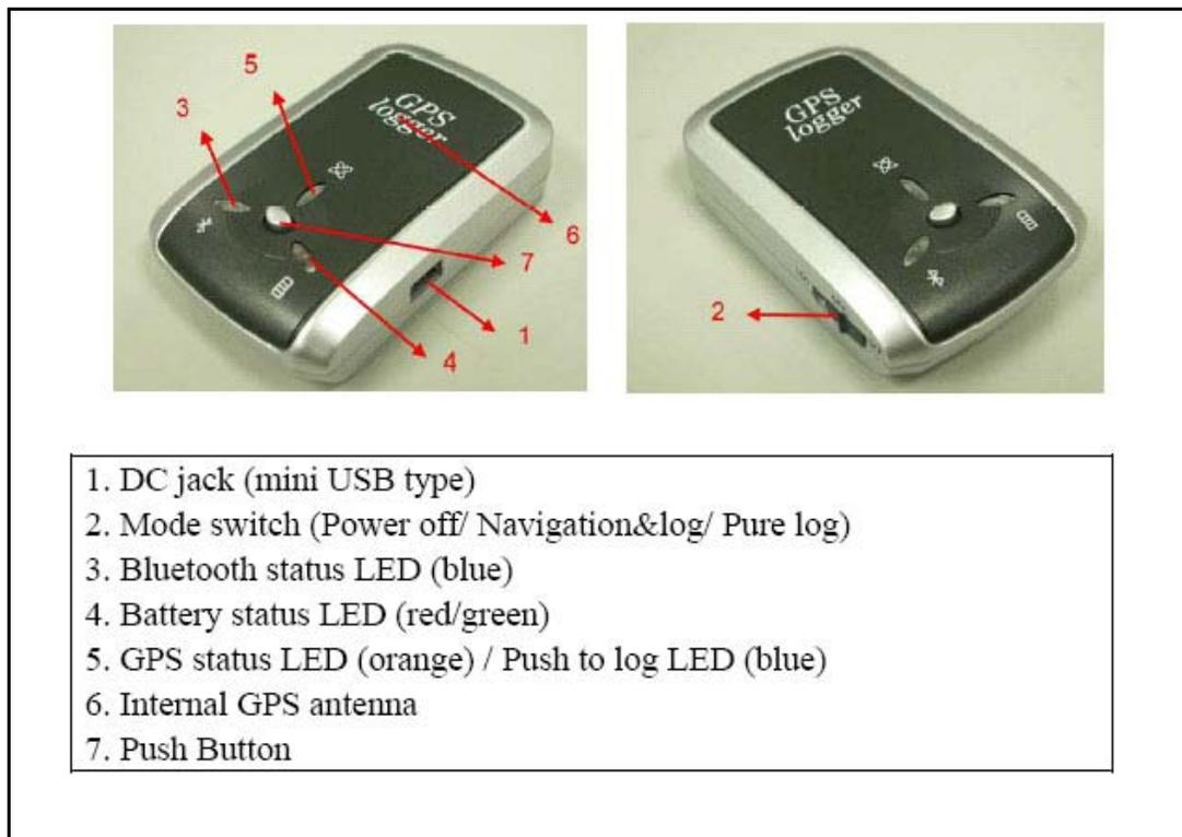
*Figure 1.1 i-Blue GPS Unit: a stream-line device, only 2” wide by 3” long*
