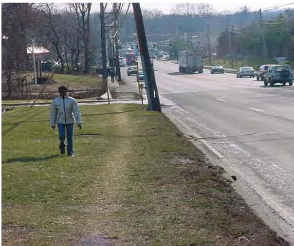
Figure 5.1 Worn Path Suggests a Sidewalk is Needed
