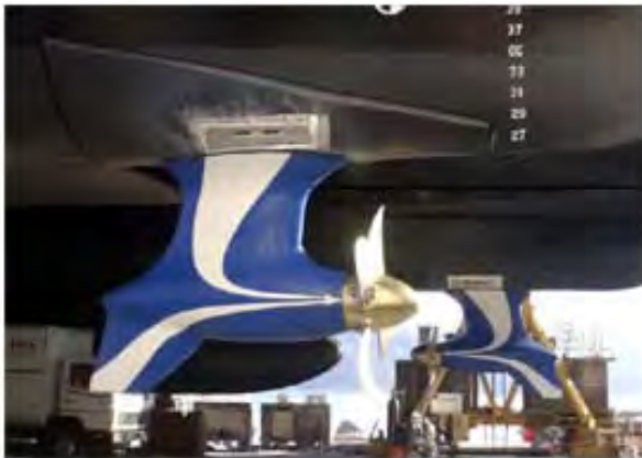
360 Degree Rotatable Thrusters and Car Deck High Enough for Trucks
