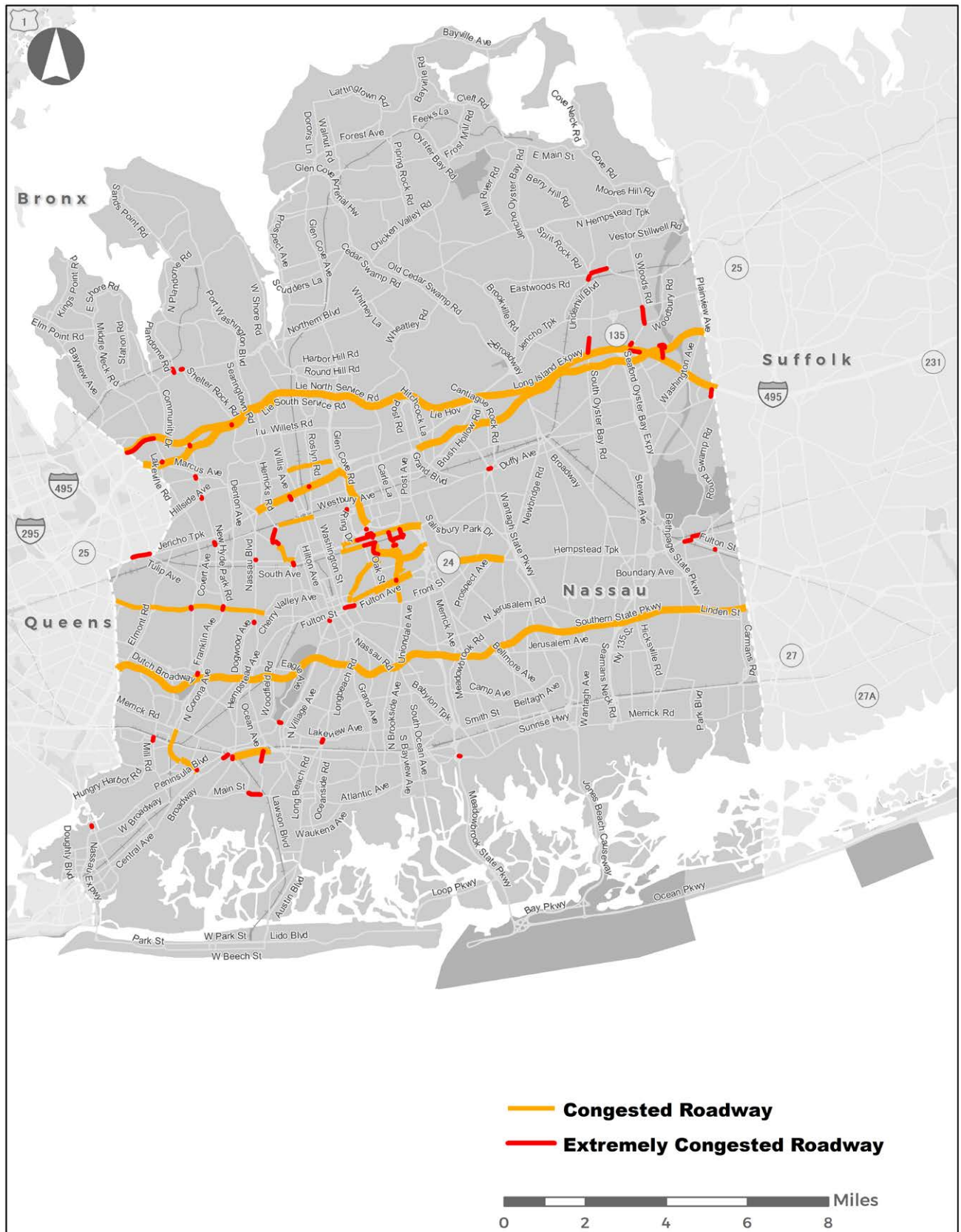
Figure A-12 Modeled Roadway Congestion for 2045 AM Peak (6 AM-10 AM), Nassau County
