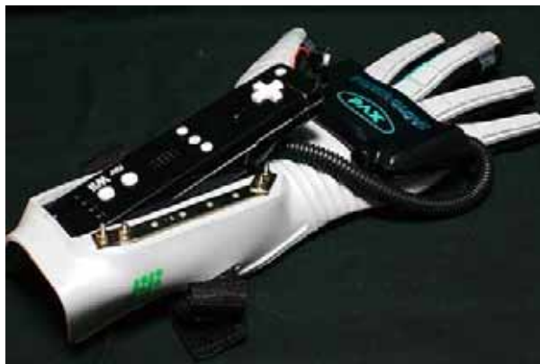
Apple iPhone and Wii Power Glove use MEMS sensors to determine orientation and hand movements.
