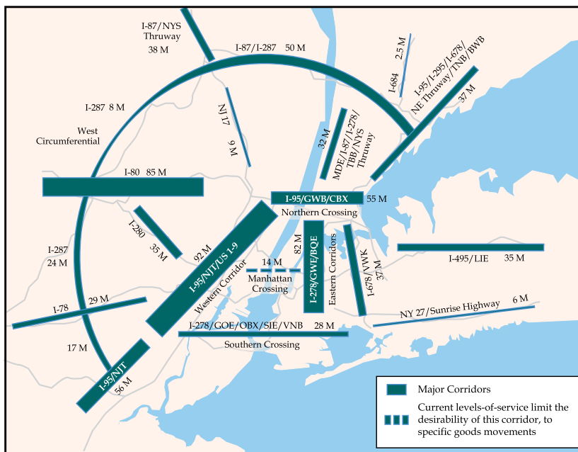
Figure 7: In this figure, the width of each line represents the volume of truck freight that moves along the indicated corridor. This means that the wider the line, the higher the volume of freight traveling along the corridor.
